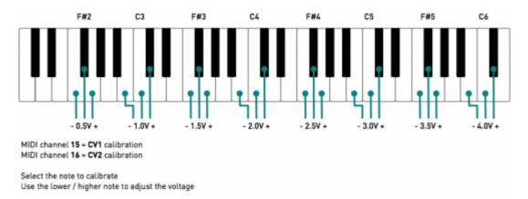
Technical note: to get maximum accuracy, it is recommended to temporarily connect a 100k resistor between the output being calibrated and ground. By doing so, the output protection resistor is taken into account. Not doing so might cause tuning errors of up to 10 cts at either ends of the scale.
